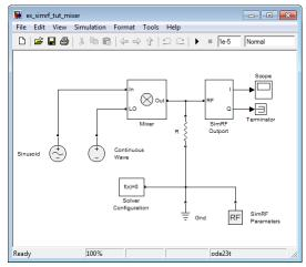
This configuration uses a SimRF Outport block as a voltage sensor at the output port of the mixer. The Simulink signal at the outport is the envelope of the carrier or carriers specified in the block. A scope attached to the outport plots the envelope. The **Output** parameter controls how signals are presented at the output ports. To change the appearance of the block, follow one of the workflows in the "Specify Block Parameters for RF Simulation" on page 2-11 section of this tutorial.
