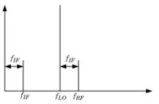
The preceding figure illustrates frequency conversion. A signal modulated on the carrier  $f_{RF}$  mixes with a local oscillator at  $f_{LO}$ . The operation downconverts  $f_{RF}$  to  $f_{IF} = f_{RF} - f_{LO}$ . The upper mixing product  $f_{RF} + f_{LO}$  is not modeled.
