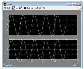
The first set of axes displays the modulation of specified carrier  $f_{IF} = f_{RF} - f_{LO}$ . This carrier appears on the first set of axes because the **Carrier Frequencies** parameter of the outport specifies it first. The second set of axes displays the modulation at  $f_{RF} + f_{LO}$ . The modulation of the upper mixing product has the same amplitude as the modulation of the downconverted signal.
