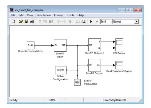
The system simulates a real passband signal as the real part of a complex passband signal according to the formula
