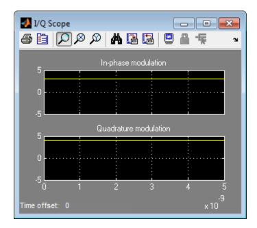
The 1-GHz carrier itself does not appear in the output. The results correspond to the real and imaginary parts of the Complex modulation at the input of the system. They also correspond to the In-phase modulation and Quadrature modulation blocks in "Simulate a Passband Signal in Simulink Software" on page 1-3.
