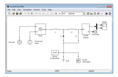
This configuration models a third-order low-pass Butterworth filter with a cutoff frequency of 1 rad/ns, or about 0.159 GHz. The high-frequency mixing product is in the stopband of the filter. The low-frequency product is in the passband.
