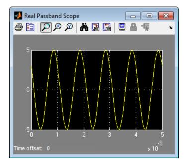
The output signal at the Real Passband Scope has a magnitude of 5 and a phase shift consistent with the specified in-phase and quadrature amplitudes.
