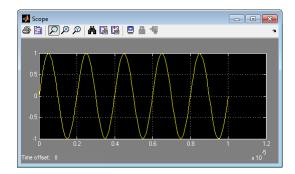
The Sinusoid specifies a 1-V amplitude for the modulation on  $f_{RF}$ , which the mixer downconverts to  $f_{IF}$ . The SimRF Outport block probes the intermediate frequency and recovers the 1-V modulation amplitude. This value agrees with a specified conversion gain of 0 dB in the mixer.
