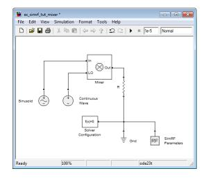
This configuration specifies an AM waveform at the input port of the mixer, an LO at the LO port of the mixer, and a  $50-\Omega$  termination at the output of the mixer.
