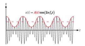
The preceding figure illustrates a signal x(t) for which circuit-envelope simulation is ideal. The signal consists of a time-varying modulation on a high-frequency carrier. In many RF applications, the frequency of the modulation A(t) is orders of magnitude less than the frequency of the carrier,  $f_c$ .
