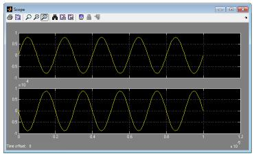
The filter attenuates the high-frequency signal at  $f_{RF} + f_{LO}$  and transmits the signal at  $f_{RF} - f_{LO}$  with minimal loss.
