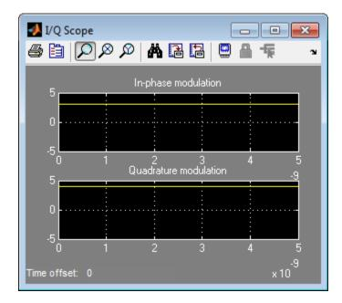
The I/Q Scope displays the in-phase and quadrature modulations of the 1-GHz signal. The 1-GHz carrier itself does not appear in the output. The results correspond to the real and imaginary parts of the Complex modulation at the input of the system.
