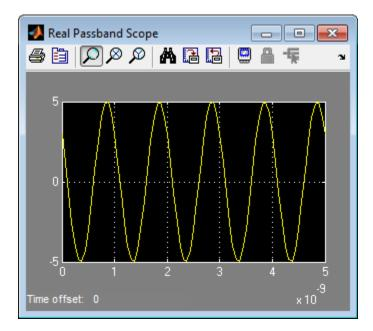
The Real Passband Scope displays the same output as the example in the previous section, "Simulate a Passband Signal in Simulink Software" on page 1-3. The signal has a magnitude of 5 and a phase shift consistent with the specified in-phase and quadrature amplitudes.
